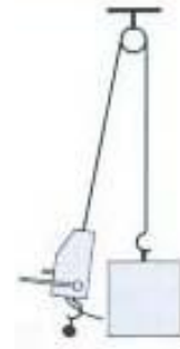
Lifting block assembly
